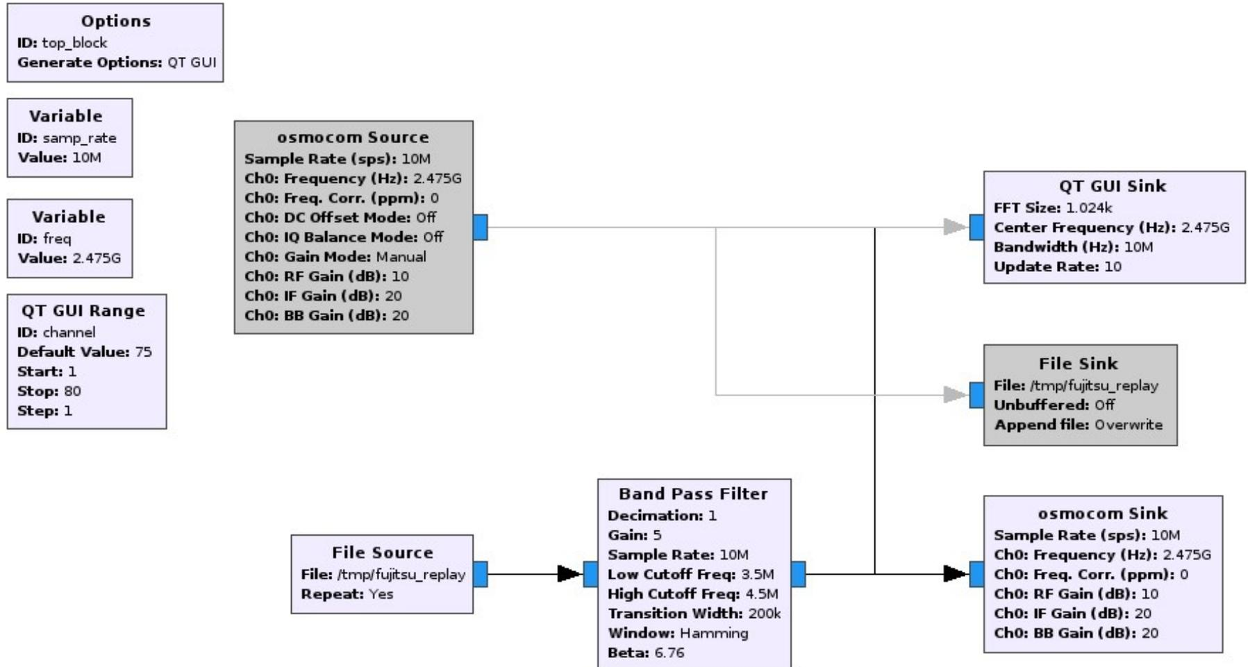
Simple GNU Radio Companion flow graph for replay attacks using a software-defined radio (HackRF One)
