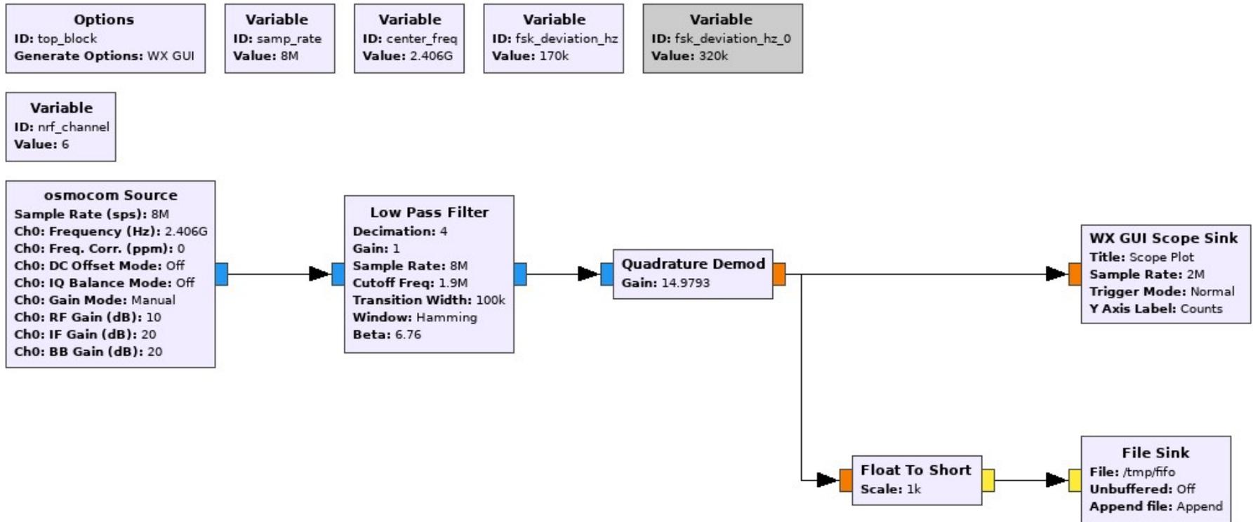
Simple GNU Radio Companion flow graph for use with modified version of NRF24-BTLE-Decoder
